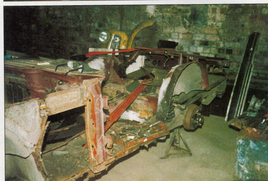
Above, a huge amount of work had to be carried out on the car's basic structure; the body was left on the chassis for this to ensure accurate panel alignment
