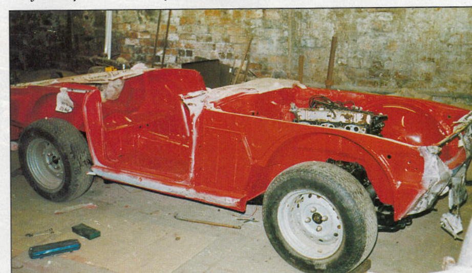
Tim practised his spraying techniques by tackling the rebuilt inner panels first
