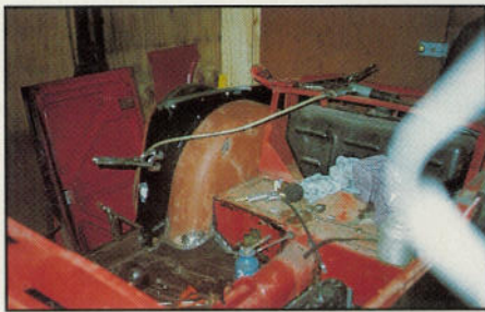
Above left, the bodysell, here primed and with sills being fitted, was completely rebuilt. Above centre, floor has been welded and new wheelarch outer panel added. Above right, new section of floor in place
