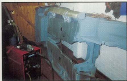
Above left, the bodysell, here primed and with sills being fitted, was completely rebuilt. Above centre, floor has been welded and new wheelarch outer panel added. Above right, new section of floor in place
