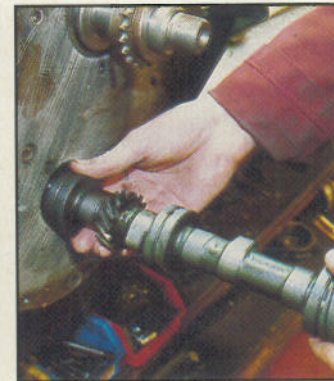
Above, Spitfire camshaft is fed into place with the engine inverted on the bench
