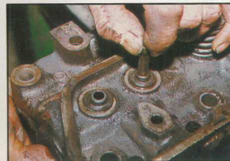
Above, deeply pitted exhaust valve seat needs to be refaced or an insert fitted. Inlet may respond to lapping
