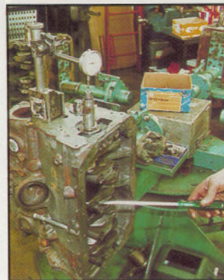
Checking crankshaft end-float, controlled by thrust washers made in different thicknesses. It should be 0.004-0.005in
