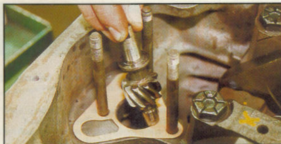
Left, using a ring compressor, the pistons are tapped in with a hammer shaft. Above, the drive pin for the oil pump is inserted. Right, the MGB's oil pump strainer is sealed to the pump body
