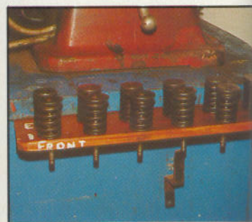
Above, it is worth making a simple wooden rack to keep the valves and valve springs in the correct order after removal from the engine
