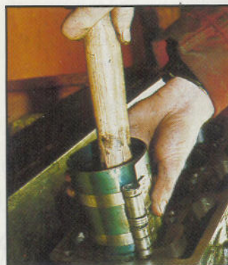
Above, after thorough lubrication, pistons are fitted using ring compressor
