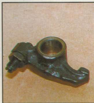
Above, bearing surface inside this rocker is badly worn and scored
