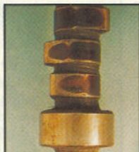
Above, a badly worn camshaft; the lobes are worn and the hardening has broken down. Left, a visual check for camshaft wear is not enough; measure it with a micrometer
