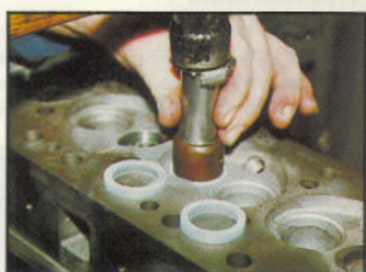
Fitting valve seat inserts. Above left, old seat machined out square. Above right, new seats, cooled in liquified oxygen, are fitted to the head, which is at room temperature. Below left, new seating being machined. Below right, check with engineers' blue shows seats do not need lapping
