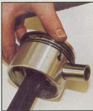
Above, Spitfire pistons may need warming to fit fully-floating gudgeon pins
