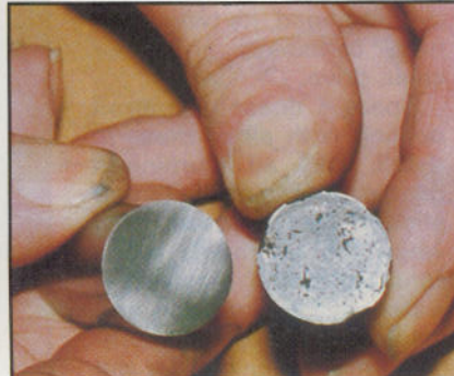
Above, serviceable tappet/cam follower on the left
