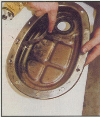
Above, this spring tensioner keeps timing chain adjusted; lubricate on assembly
