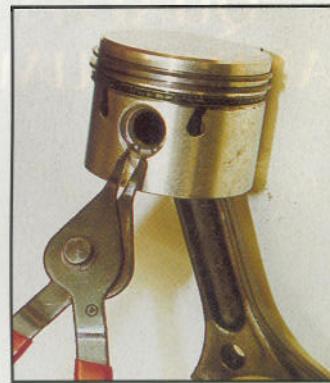
Above, gudgeon pins are secured in the piston by Seeger circlips
