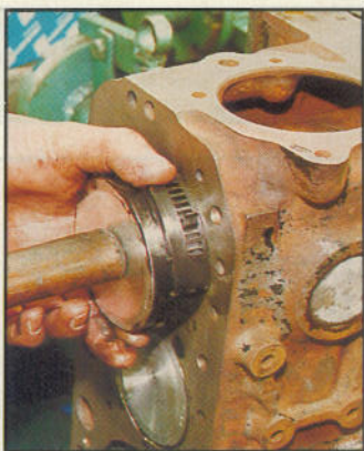
Left, using a ring compressor, the pistons are tapped in with a hammer shaft. Above, the drive pin for the oil pump is inserted. Right, the MGB's oil pump strainer is sealed to the pump body
