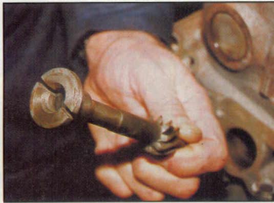
Above, serviceable tappet/cam follower on the left
