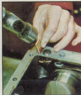
Above, sealing block fitted and wooden packing being tapped in
