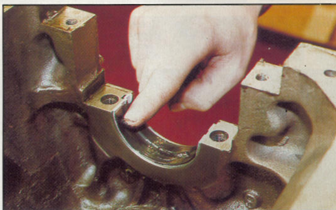
Above, Spitfire's rear crankshaft seal track must be lubricated generously. Right, sealing block and packing (front) and rear seal housing and gasket
