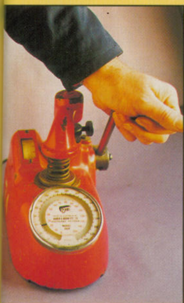
Left, testing a valve spring in a proper professional rig which gives a read-out of poundage
