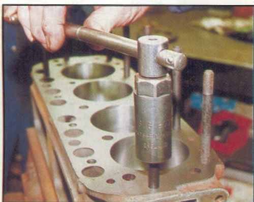
Left, fitting head studs; there are two lengths, long ones go on the nearside. Above, jointing compound being applied to head gasket; card avoids sticky fingers. Right, oiling pushrods before fitting rocker assembly
