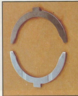
Above, thrust washers. The grooved whitened side (bottom) must be towards the crankshaft
