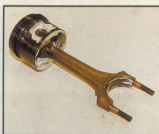
Above, piston ring gaps are staggered. Piston and shell bearing have been lubricated with Graphogen grease
