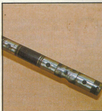
Above, worn rocker shaft: locating groove and oil feed (centre), choked oil drilling to rocker on right
