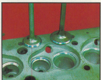
Fitting valve seat inserts. Above left, old seat machined out square. Above right, new seats, cooled in liquified oxygen, are fitted to the head, which is at room temperature. Below left, new seating being machined. Below right, check with engineers' blue shows seats do not need lapping
