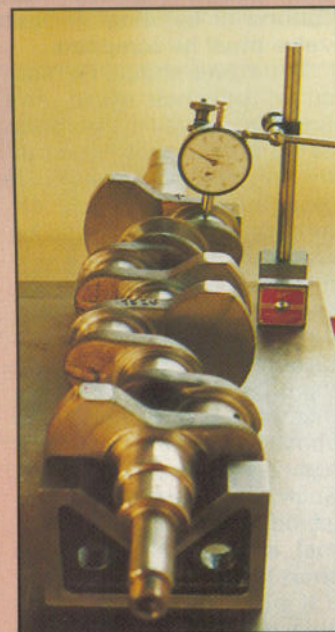
Testing crankshaft for twist. Both end crankpins should be the same height from surface table, as shown by dial gauge
