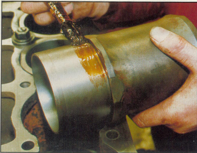
Above, the cleaned seatings on the bottom of the liners and in the block are painted with Wellseal
