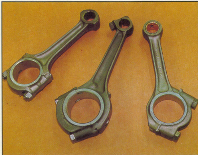
Above, it is vital to number big-end bearing cap and connecting rod before dismantling, to ensure that the cap goes back on the same rod and is the right way round on reassembly
