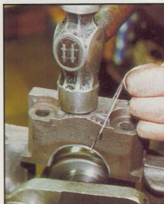
Above, fitting rear main bearing cap. The string prevents the shell falling as the cap is tapped home
