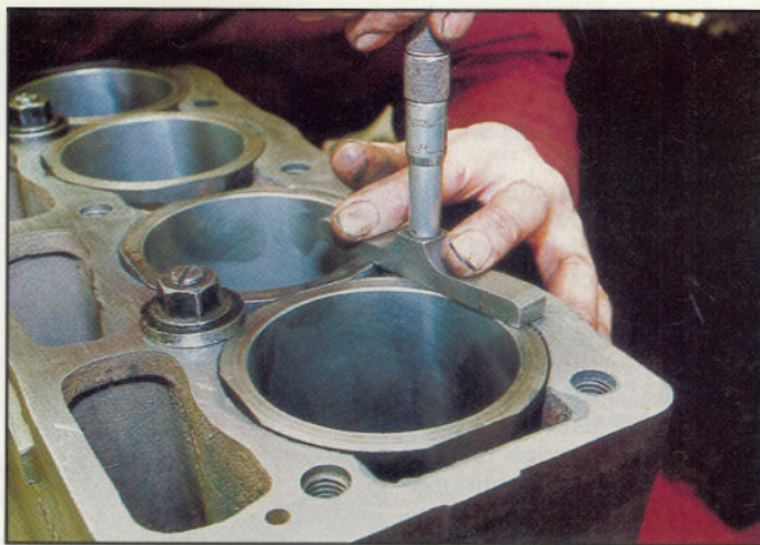
Above, after assembly with new gaskets, each pair of liners is secured by a short stud with a nut and heavy washer. Here a micrometer depth gauge is being used to check liner protrusion, which should be 0.0035-0.005in Below, the front bearing/sleeve controls camshaft end-float
