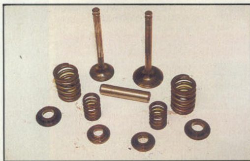
Above, Triumph Spitfire valves, exhaust on the left and larger inlet on the right
