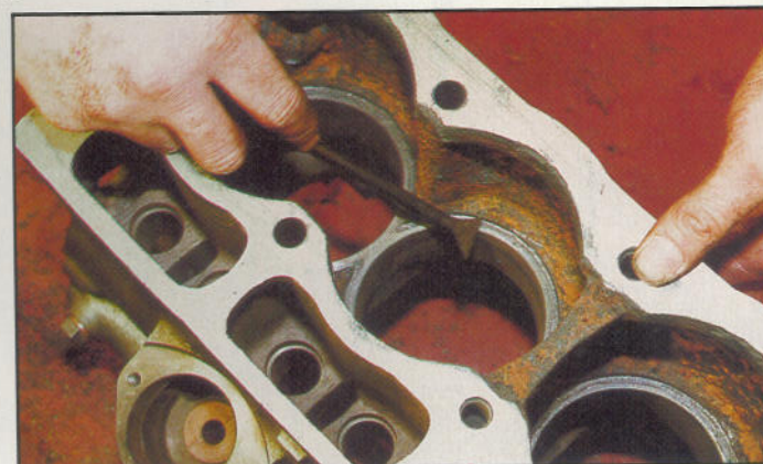
The bottom seating for the liners must be clean, flat and smooth. Here the remains of an old liner gasket are being carefully scraped away
