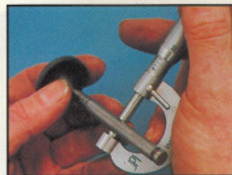
Measuring the diameter of a valve stem with a micrometer
