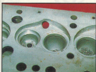
Fitting valve seat inserts. Above left, old seat machined out square. Above right, new seats, cooled in liquified oxygen, are fitted to the head, which is at room temperature. Below left, new seating being machined. Below right, check with engineers' blue shows seats do not need lapping
