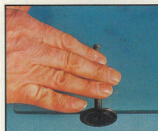
Above, rolling valve on plate glass to test for bending
