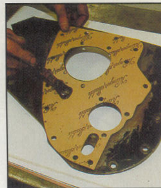
Above, preparing Triumph Spitfire front engine plate for fitting
