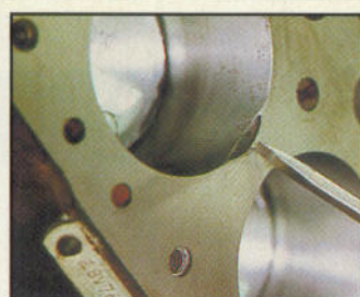
Above, piston ring gaps must be positioned away from this cutout when the pistons are fitted into the bores
