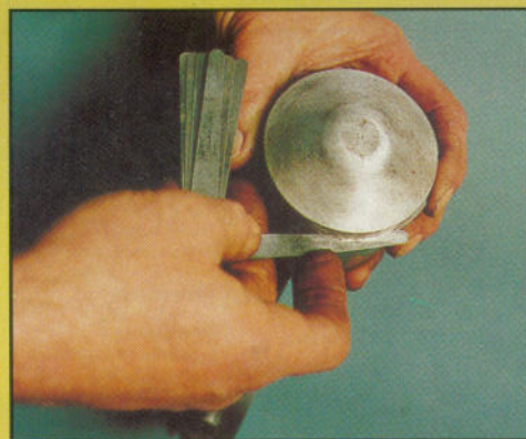
Left, testing piston ring side clearance using a feeler gauge
