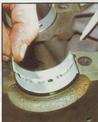
Above, fitting main bearing shells. Engage lugs in their 'nibs' and push the shells home
