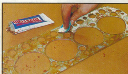
Left, fitting head studs; there are two lengths, long ones go on the nearside. Above, jointing compound being applied to head gasket; card avoids sticky fingers. Right, oiling pushrods before fitting rocker assembly
