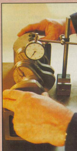
Testing crankshaft for 'bow'. Gauge mounted at centre main journal should show steady reading when shaft is turned
