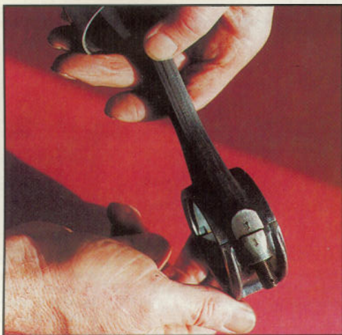
Above, it is vital to number big-end bearing cap and connecting rod before dismantling, to ensure that the cap goes back on the same rod and is the right way round on reassembly
