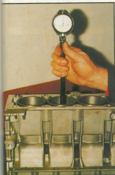
Below, measuring cylinder bore wear using a comparator gauge
