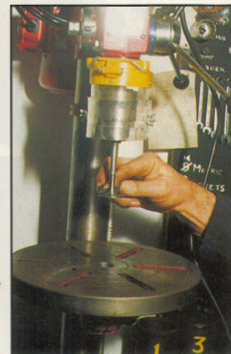
Measuring the diameter of a valve stem with a micrometer
